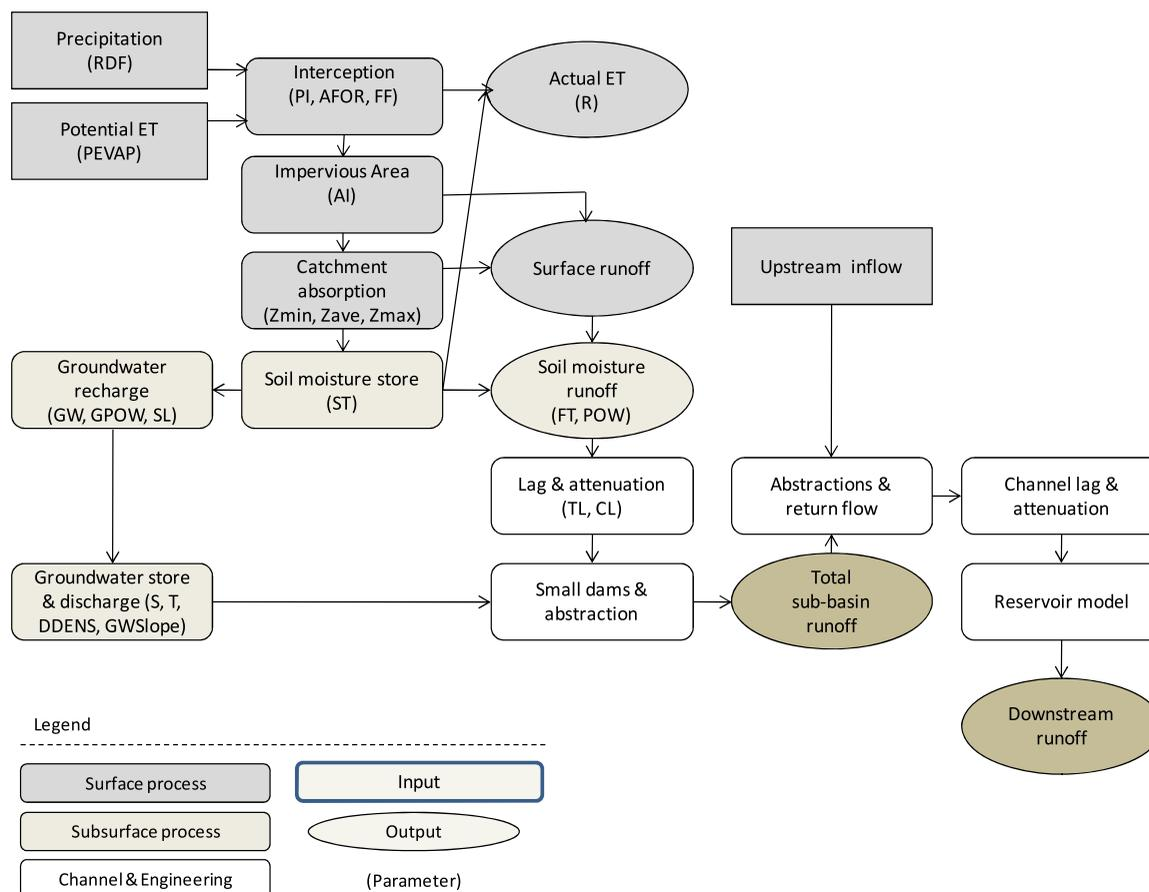
Figure 3. Flow diagram of the GW-PITMAN model showing the main model components and their relevant parameters [Kapangaziwiri, 2010].
