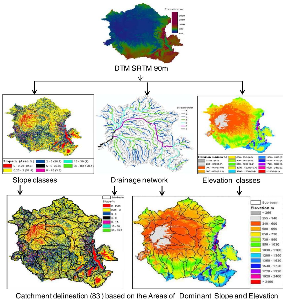
Figure 2. Spatial characteristics and modeling units (subbasins) of the Congo Basin based on the SRTM data set.
